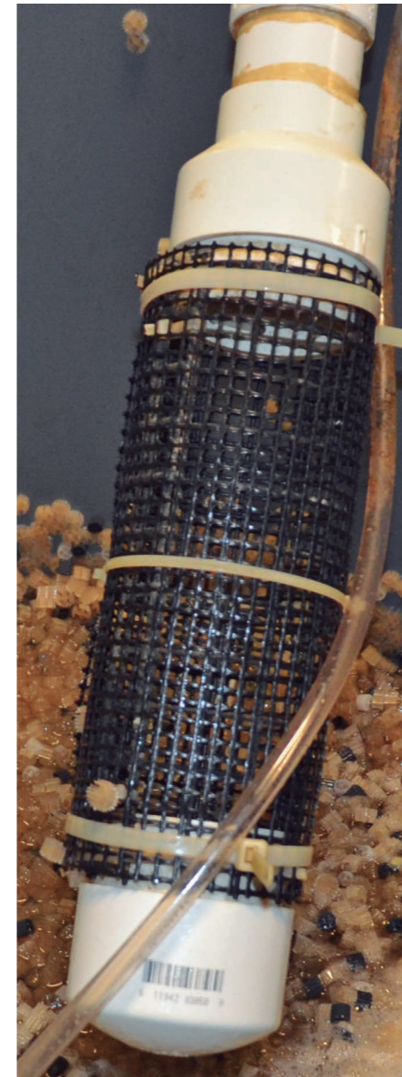
Figure 6. A screened outflow in a biofilter. This can be placed on the tank bottom to allow water to pass through but not bio-media. Also note the small bio-media, most of which has turned brown, indicating a population of helpful bacteria is established.
