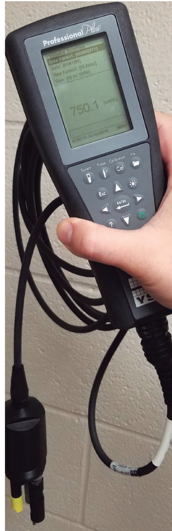
Figure 9. A multi-parameter water quality instrument. This unit measures temperature, pH, DO, salinity, conductivity, and barometric pressure. This type of device is expensive but it measures some of the most critical life-sustaining parameters.
