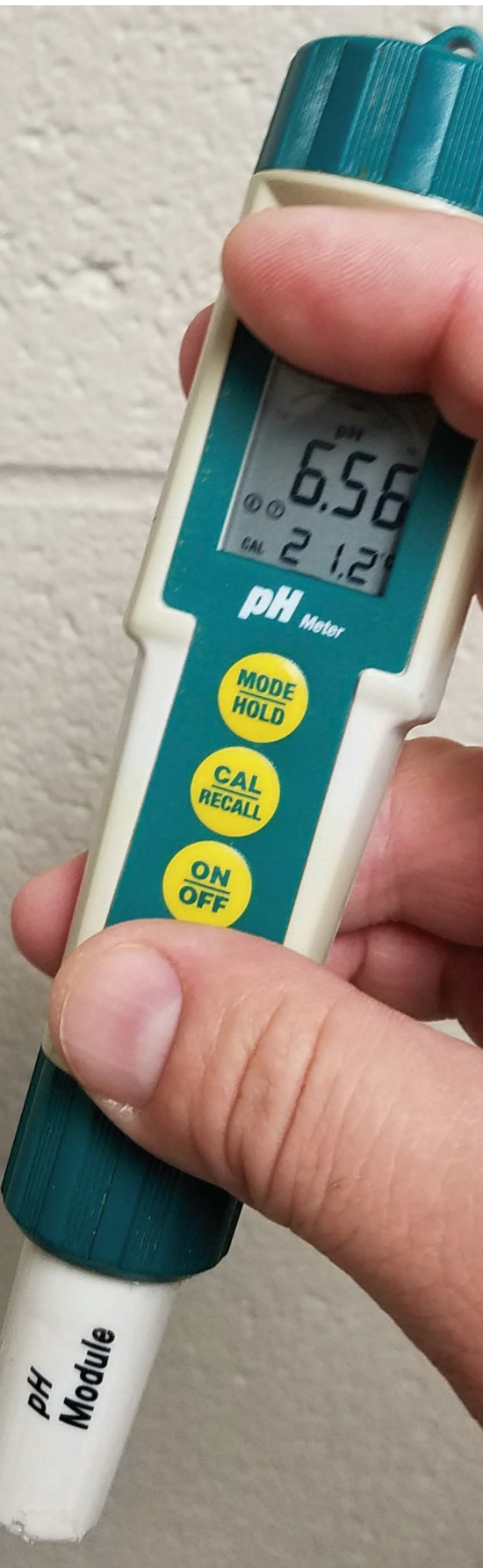
Figure 10. A pH and temperature meter. This type of meter is much less expensive than a multi-parameter style unit. Similar instruments can measure DO and salinity.
